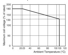
**Note:** The maximum coil voltage refers to the maximum value in a varying range of operating power voltage, not a continuous voltage.
